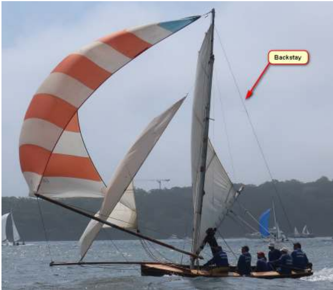
Backstay from the top of the gaff to the transom
