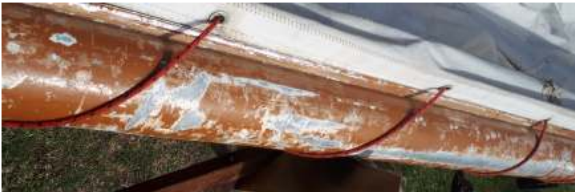
Mainsail laced to the boom using round lashing
