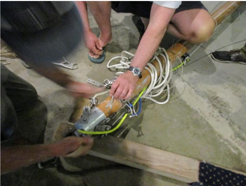
Jack Tang, Jamie Watt and Greg Kay examining the damaged jib halyard fitting that cost Scot the lead in the final race of last season.
